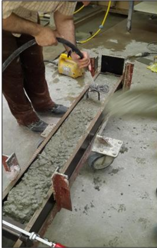
Figure 9: Confection des poteaux.
