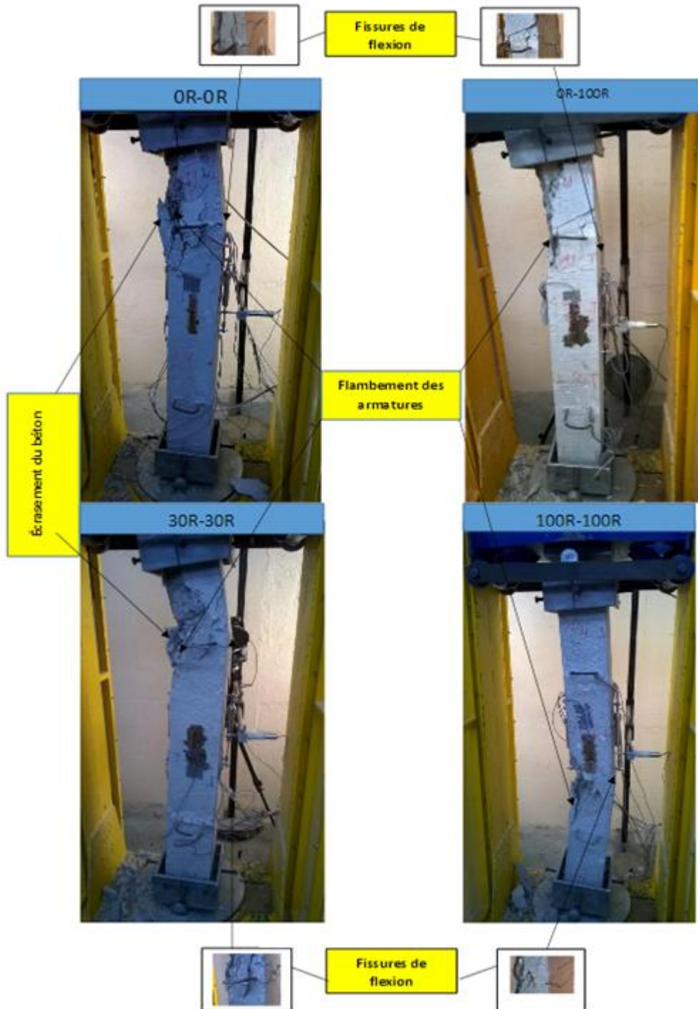
Figure 24: Essai de compression excentrée
