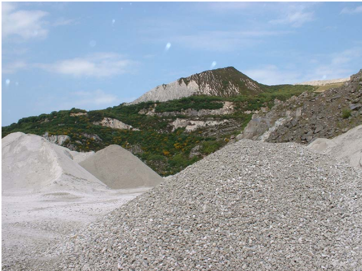
Figure 1 Photograph showing production stockpiles of china clay waste (foreground and mid-ground left), uncrushed stent still on the quarry face (mid-distance right) and an old spoil heap (far distance)
